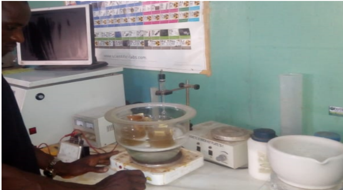
Figure 1: Depositing Precursor Solution in a water bath during film growth.
