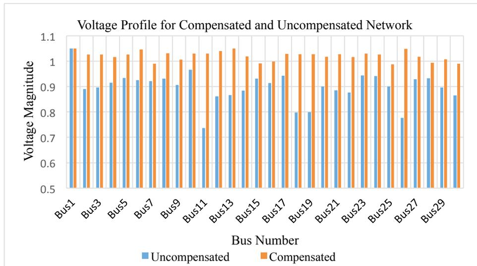
Fig.2. Voltage amplitude before and after compensation.
