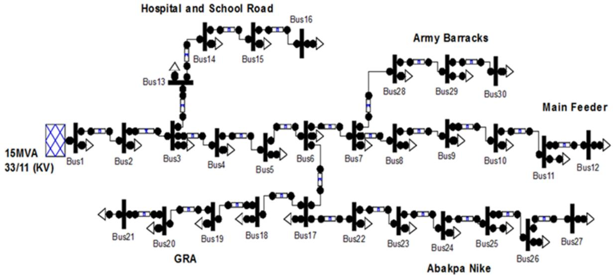
Fig. 1: Single line diagram of Thinker's Corner distribution feeder.
