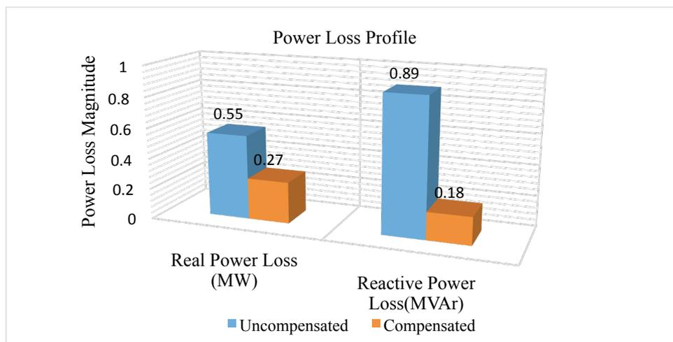
Figure 3: Power loss before and after compensation
