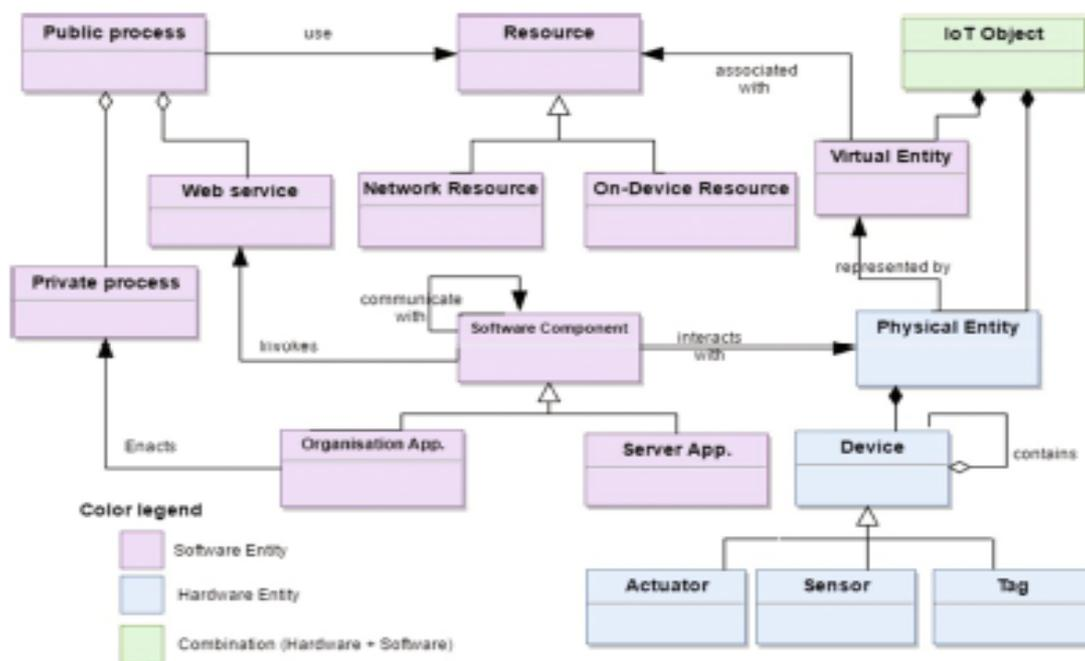
Fig. 1. Domain model of health institution application based on IoT
