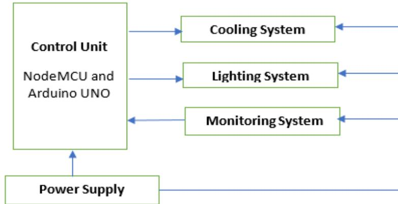
Figure 2: Block diagram of the hardware system
