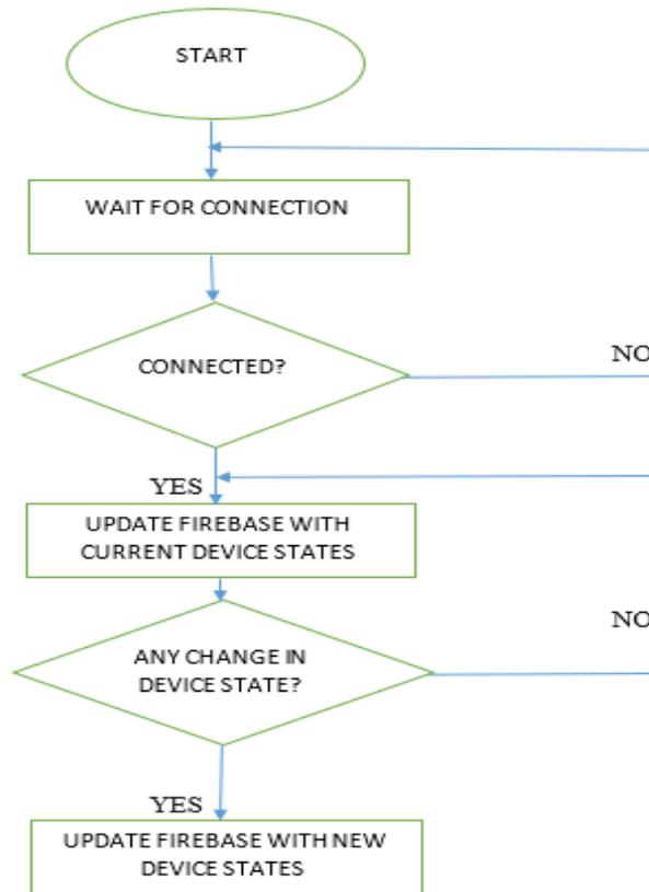
Fig 7: The software flow diagram
